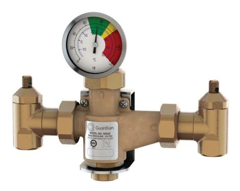
**Application:** Thermostatic mixing valve to blend hot and cold water to deliver tepid water. Valve has flow capacity of 13 gallons (49 liters) per minute at 30 PSI (2.1 bar) pressure drop. Valve can be used to supply emergency eyewash, eye/face wash or drench hose unit. Depending on water supply size and pressure, valve can supply multiple units.
