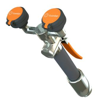
**Application:** Dual purpose eyewash/drench hose unit for 45 degree angled panel mounting. Unit meets the provisions of ANSI Z358.1 -2014 as both an eyewash and a drench hose. Unit may be left in the angle holder for use as a fixed eyewash, leaving user's hands free. Alternatively, unit may be removed for use as a drench hose to rinse any part of user's eyes, face or body.
