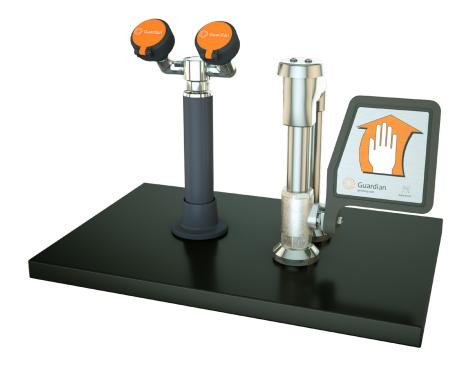
**Application:** Dual purpose eyewash/drench hose with ball valve and flag handle for deck mounting. Unit meets the provisions of ANSI Z358.1-2014 as both an eyewash and a drench hose. Unit may be left in the deck flange for use as a fixed eyewash, leaving user's hands free. Alternatively, unit may be removed for use as a drench hose to rinse any part of user's eyes, face or body. Vacuum breaker prevents external water and contaminants from seeping back into supply line.
