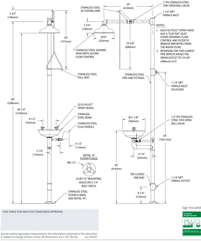
Guardian Equipment 1140 N North Branch St Chicago, IL 60642 312 447 8100 TELEPHONE 312 447 8101 FACSIMILE gesafety.com Listed 8116. Units have been tested to and comply with ANSI Z358.1-2014 and the Uniform Plumbing Code.
