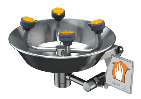
**Application:** WideArea<sup>™</sup> eye/face wash for wall mounting. Constructed entirely in stainless steel. Ideal for use in highly corrosive environments and cleanroom applications. Four GS-Plus™ spray-type outlet heads deliver a flood of water over a wide area of coverage for complete rinsing of eyes and face.
