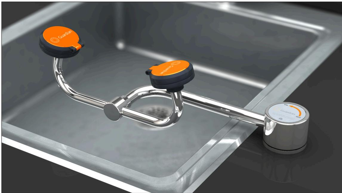
**Application:** AutoFlow™ eye/face wash for mounting on counter next to sink. Swinging the spray head assembly 90 degrees horizontally out over sink activates the water flow. The unit remains in operation until the spray head assembly is swung back into the storage position, closing the valve.
