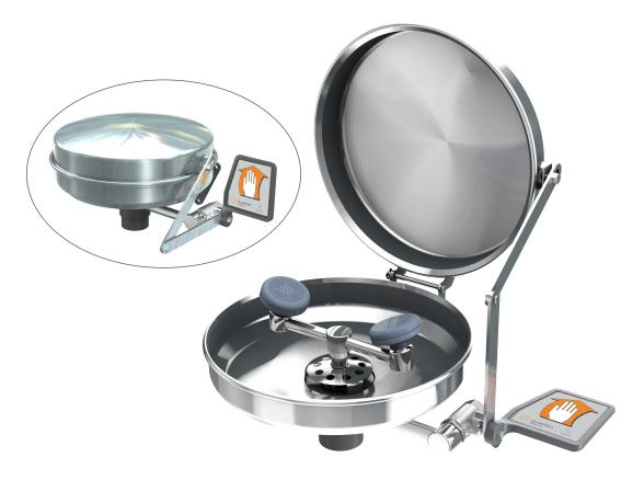
**Application:** Eye/face wash for wall mounting. Unit has stainless steel cover to protect bowl from dust, dirt and other contaminants. Two large FS-Plus™ spray-type outlet heads deliver a flood of water for rinsing eyes and face.
