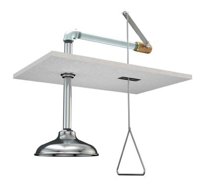
**Application:** Emergency shower for semi-concealed mounting in a finished ceiling. Unit is designed for installation in ceilings 8-10 feet above finished floor.
